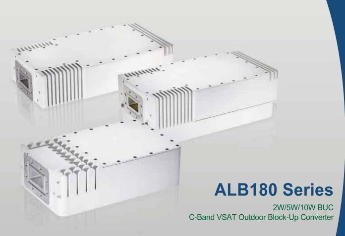
Agilis ALB180 K-Series C-Band BUC (Block-up Converter) is a highly cost effective outdoor RF transmitter for satellite communication. The BUC has very high output power linearity and works well from -40°C up to 60°C. The BUC also has a wide input voltage range which allows it to work from 18V to 60V for 5W and 10W models.
